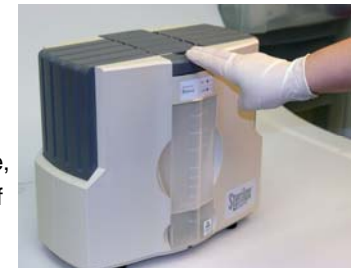
Press the Dispense Button to generate Sterilox Solution for priming.
