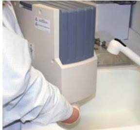
Empty the reservoir tank of all residual Sterilox Electrolyte Solution.
